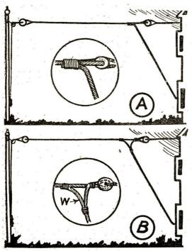
The wrong way, A, and the correct way. B to attach your down-lead.
