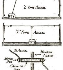
Fig. 2.—Two very efficient aerials and lead-in.
